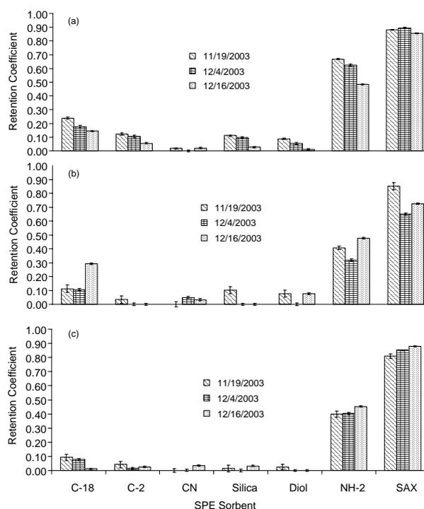
Fig. 2. RCs for the (a) pilot plant influent, (b) CF effluent and (c) CF-O<sub>3</sub>/BF effluent.
