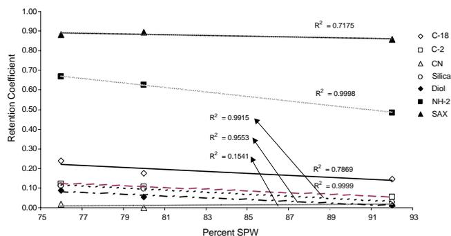
Fig. 3. Linear regressions showing the relationship between RC and the percent SPW in the influent water.  $R^2$  values closer to 1.0 indicate variability in the percentage of SPW better explains the RC variability for a particular resin.
