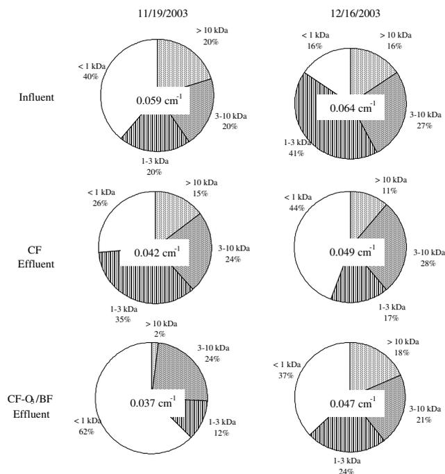
Fig. 6. Pie charts for two sample dates show temporal differences in the influent UV<sub>254</sub> size distribution and how the CF-O<sub>3</sub>/BF and CF treatment trains changed the size distribution. The sample dates are included at the top of the graphs and the sample sites are listed to the left. Results are shown as a percentage of the total UV<sub>254</sub> (shown in the center of each pie chart) for the given sample site on the indicated date.
