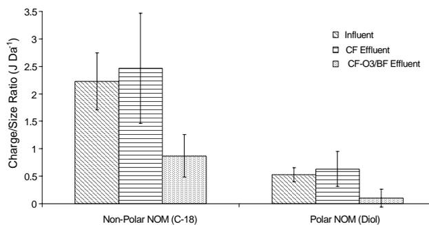
Fig. 7. Average  $\Delta E^i/MW$  ratio in terms of  $\Delta E^i$  (J) and MW (Da) for non-polar and polar NOM at the pilot plant influent and the effluent of each treatment train. The Hansen solubility parameter for C-18 and Diol SPE resins were used to determine the  $\Delta E^i/MW$  ratio of the non-polar and polar components of the NOM, respectively. Error bars represent the standard error for these data.
