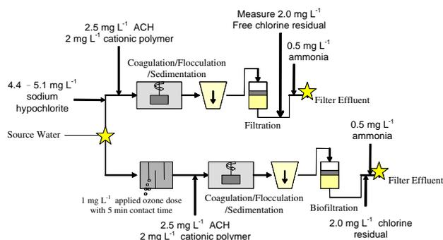
Fig. 1. Process diagram for CF (top) and CF-O<sub>3</sub>/BF (bottom). The stars indicate water quality and NOM sample collection sites.
