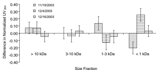
Fig. 5. Normalized size fraction data for CF-O<sub>3</sub>/BF effluent subtracted from CF effluent. Positive values indicate the CF effluent had a higher UV<sub>254</sub> for a particular fraction than CF-O<sub>3</sub>/BF effluent. The opposite is true for negative values.
