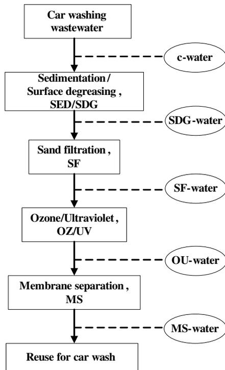
Fig. 1. The treatment processes of the car wash wastewater.
