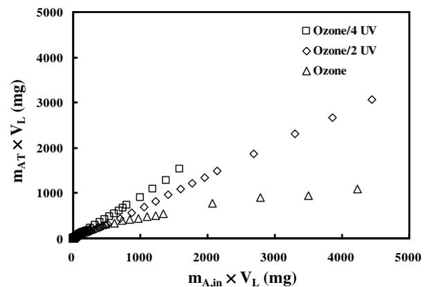
Fig. 3. Gaseous ozone transferred dosage (m<sub>AT</sub> × V<sub>L</sub>) vs. m<sub>A,in</sub> × V<sub>L</sub> for various ozonation processes. m<sub>AT</sub>: Defined in Eq. 2. V<sub>L</sub>, 2 UV and 4 UV: As specified in Fig. 2.
