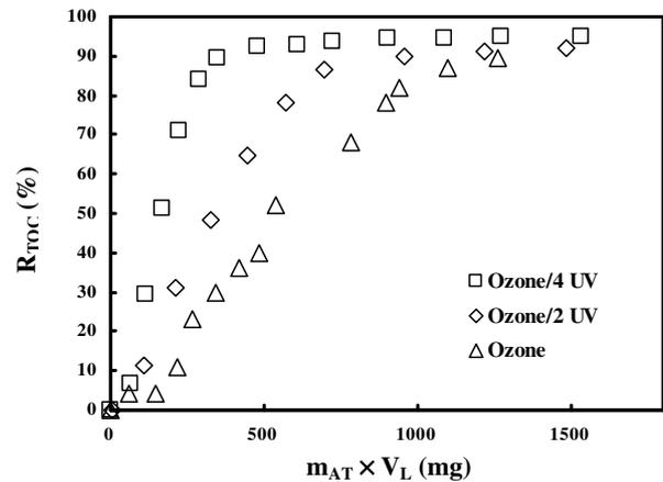
Fig. 2. Removal efficiency of TOC (R<sub>TOC</sub>) vs. gaseous ozone applied dosage (m<sub>A,in</sub> × V<sub>L</sub>) for various ozonation processes. m<sub>A,in</sub>: Defined in Eq. 1. Volume of water (V<sub>L</sub>) = 4 L. 2 UV, 4 UV: Using 2 and 4 UV lamps with total powers of 13.92 and 27.84 W, respectively.
